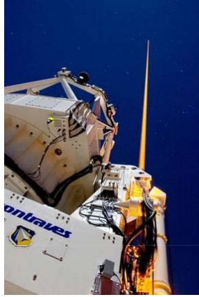
Figure 12. 3.5m telescope at the Starfire Optical Range near Albuquerque, NM. with side launched laser[27].
